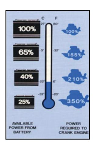
As you can see from this chart, a fully charged battery at 80° has 100% of its starting power capacity.
